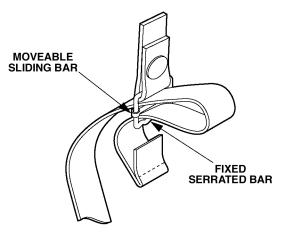
Figure 3-2. Threading the Sliding Bar Buckles.
